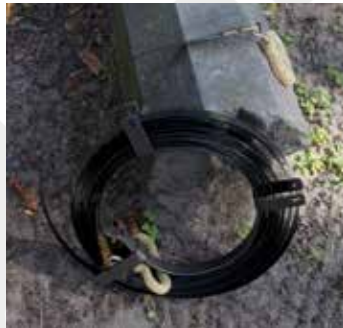
83.4 Surveying tape or classic geodetic tape. Decimetre divisions are marked with holes, e.g. every 0.5 m is a rivet, and every 1 m is a metal plate marking full metres. The tape comes with a special handle for easy transport and winding. Today, this equipment has been almost completely replaced by modern measuring methods.
