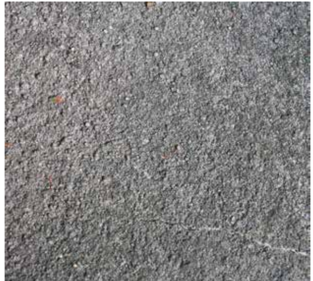
ILL. 54 Concrete with clearly visible sand grains
